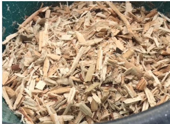
Figure 2 Water hyacinth fibers grinded through 1 inch of sieve size.
