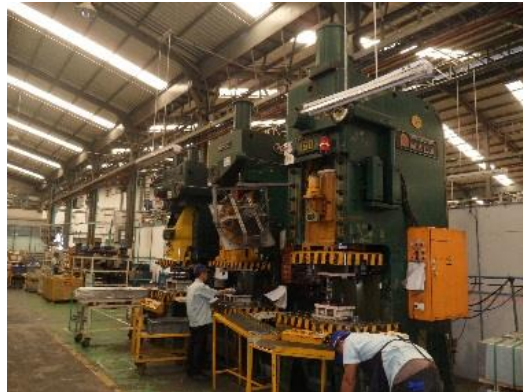
Figure 1 The 500 tons forming machines used in the test.
