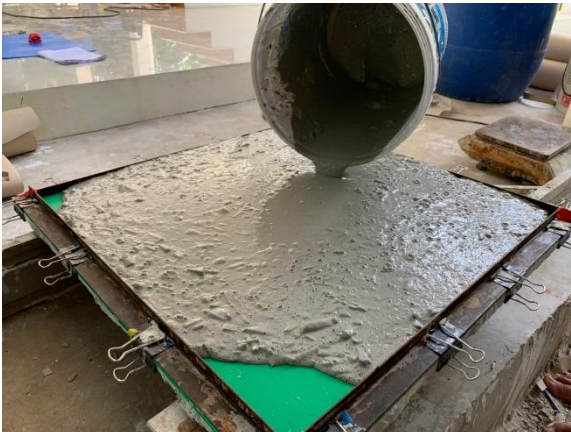
Figure 3 Pouring the mixture into the mold.
