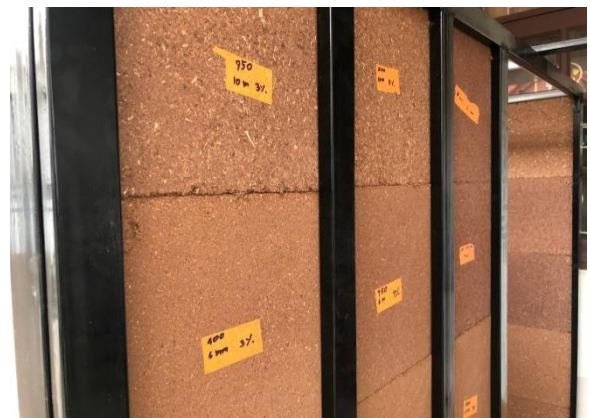
Figure 16 The decoration of particleboards from eucalyptus bark.
